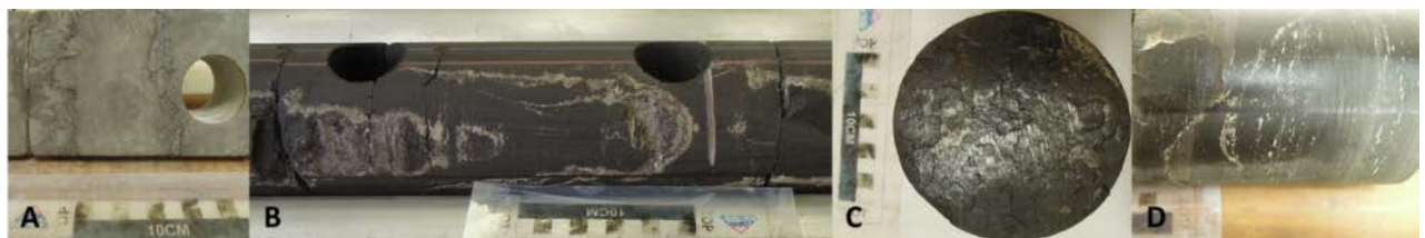
Figure 1 - Examples of features: A - Sedimentary Stylolites; B – En-echelon partially open fractures with calcite filling; C – Surface of a Stratification Gliding Plane with respective striation; D – Fault.
